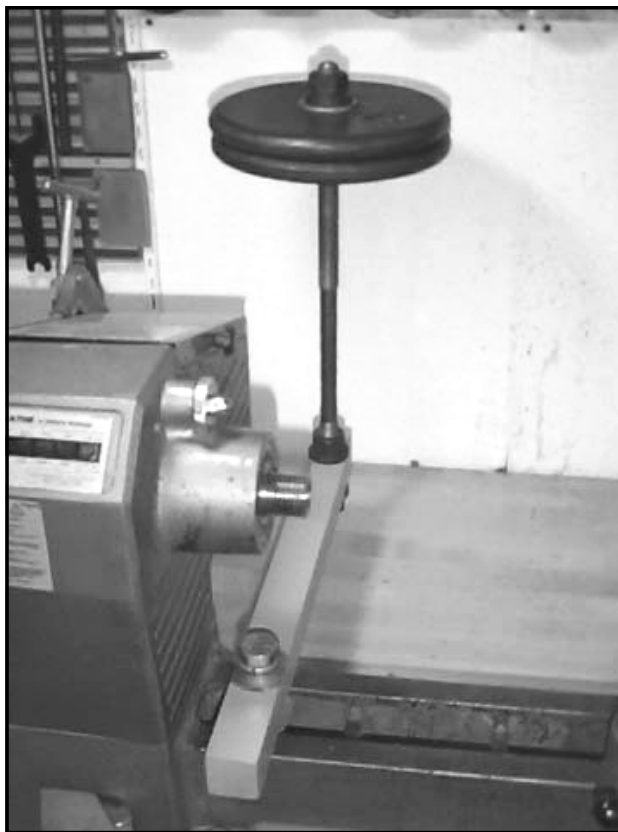
The Glaser TVA is shown here bolted to the bed of the author's Nova 3000.
