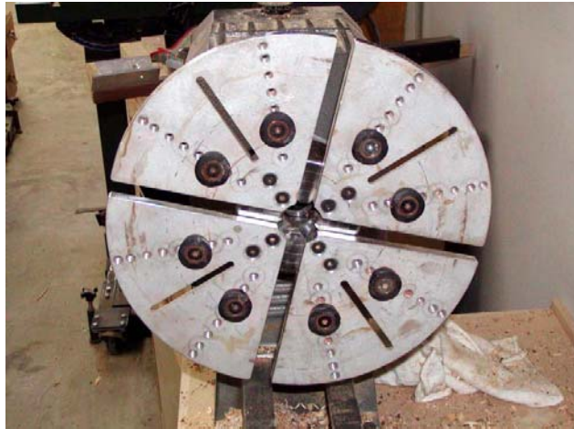
Photo 1. A Chuck with mounted Cole Jaws.
