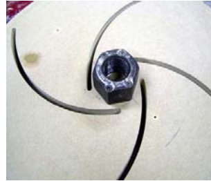
Photo 6. This photo shows the routed arcs on the reverse side of the chuck base plate and the nut that was used instead of a faceplate.
