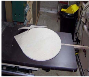
Photo 5. Circle cutting jig makes cutting the disks easy.
