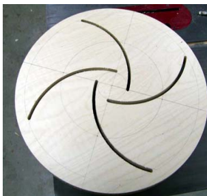
Photo 11. The arcs have been routed.
