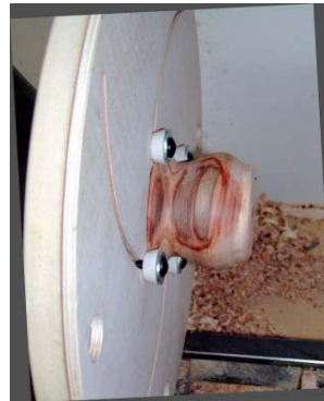
Photo 3. This photo shows the Author's Longworth Chuck holding a small bowl. The chuck is very versatile.
