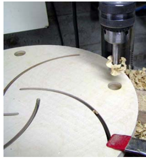
Photo 12. Drilling the Finger Holes near the rim of the disks.
