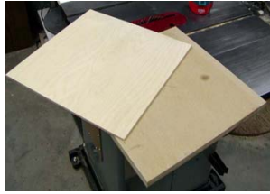
Photo 4. Recycled scraps of 3/4" MDF and 1/4" Birch Plywood to use in making the disks.
