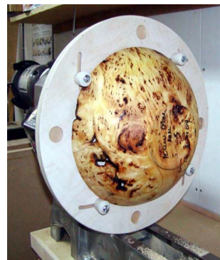
Photo 2. This photo shows the Author's new Longworth chuck holding a bowl for turning the foot.
