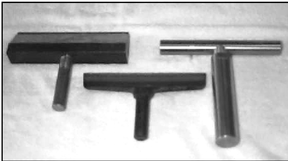
This photo compares three six inch tool rests and shows their relative size. (From left to right): Woodcraft, Jet Mini, and BestWoodTools, with a larger 1 inch post).
