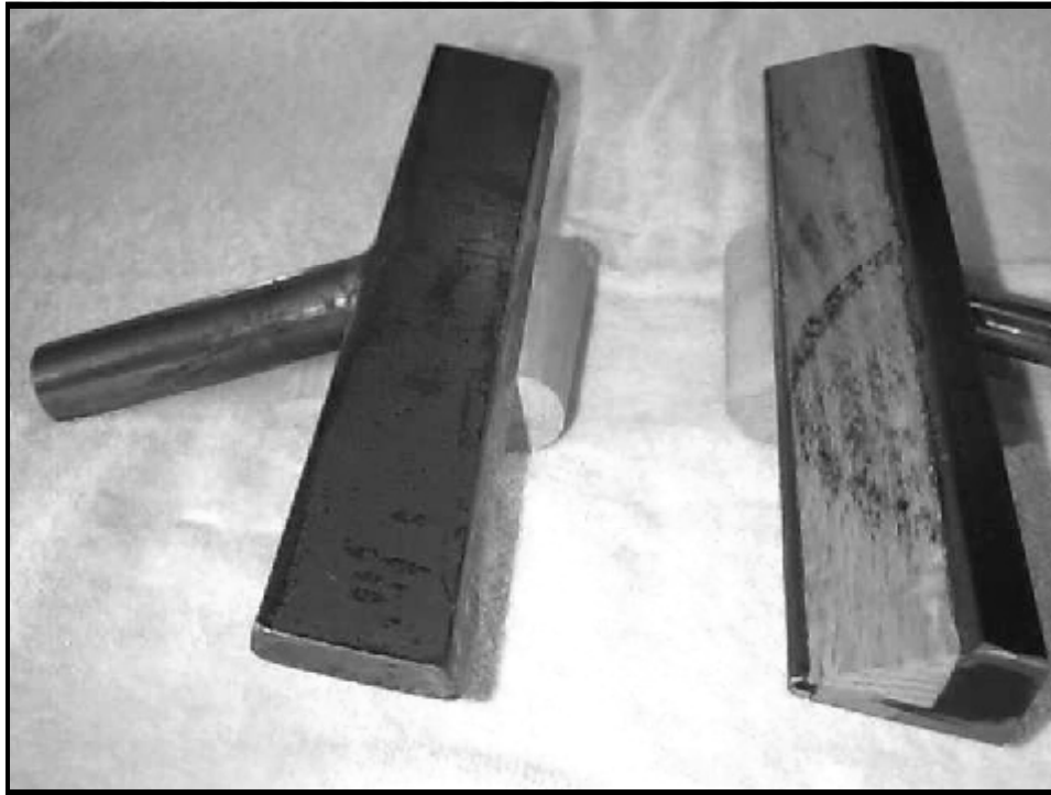
This view compares the stock 12 inch Nova 3000 tool rest (left) to the 12 inch replacement tool rest from Woodcraft. Note the extra width at the body of the Woodcraft.
