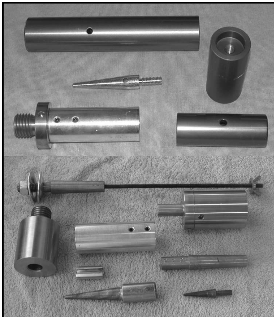
Various methods of mounting buffing wheels to the lathe.
