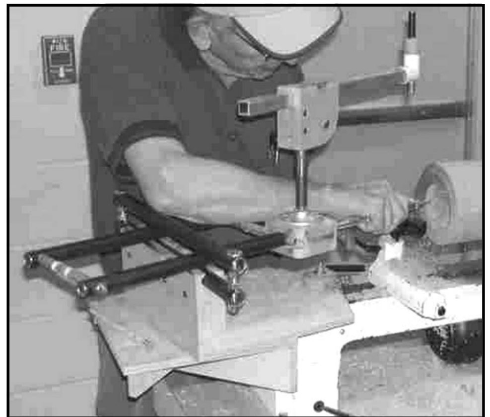
Home built hollowing rig with laser for a mini-lathe.
