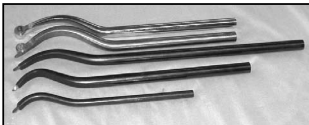
A selection of curved tools in the Author's tool inventory: (from the top) 1) Don Pencil Scorpion; 2) Dennis Stewart Hooker; 3) Jordan 3/4" Large Curved; Jordan 3/4" Medium curved; and Jordan 1/2" curved.
