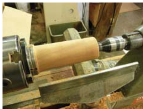
Figure 1. Here the wood has been turned round and to about 1-1/2" in diameter.
