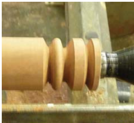
Figure 3. Here the top of the ring to be has been cut with the Sorby beading tool.
