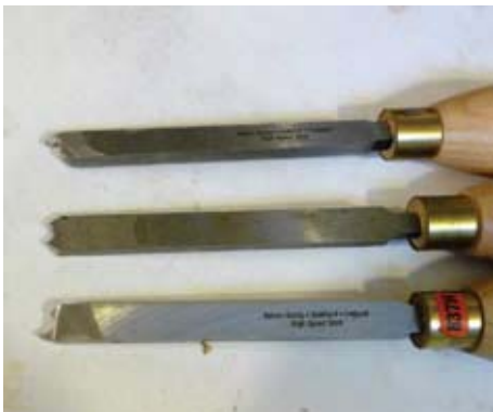
Figure 7. The Robert Sorby tools used in this project: (top to bottom) Right hand side tool, beading tool, and left hand side tool.
