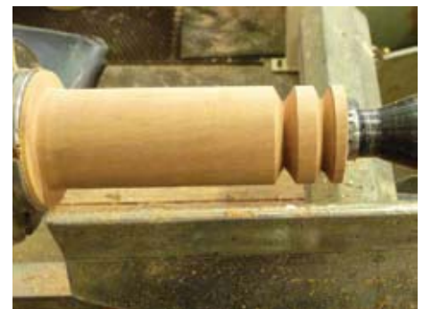
Figure 2. Two V-cuts have been made near the tailstock. The space in between the cuts will define the knob on the end for teething.
