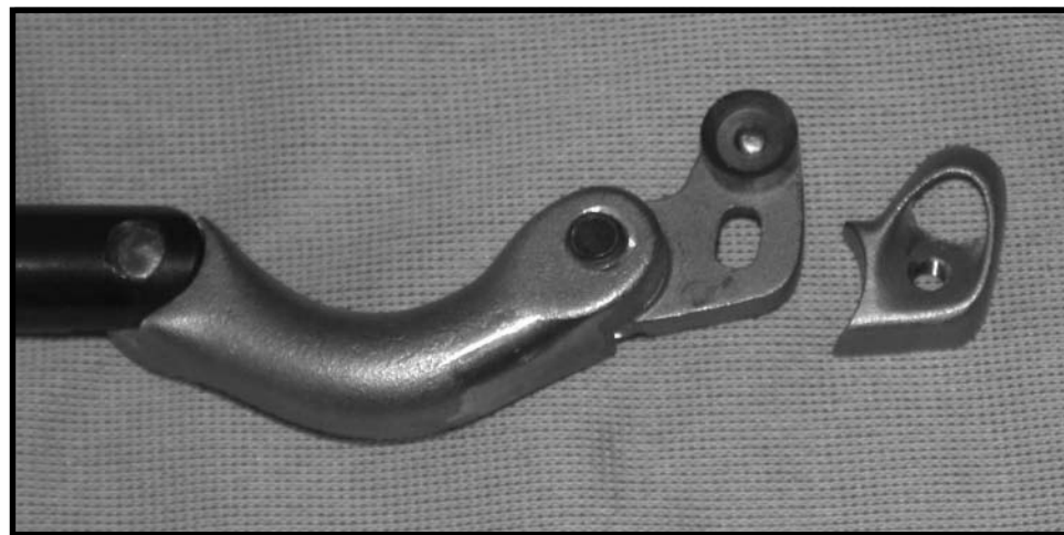
This view shows the business end of the Munro Hollower in the position for cutting. the stainless steel hood has been removed.
