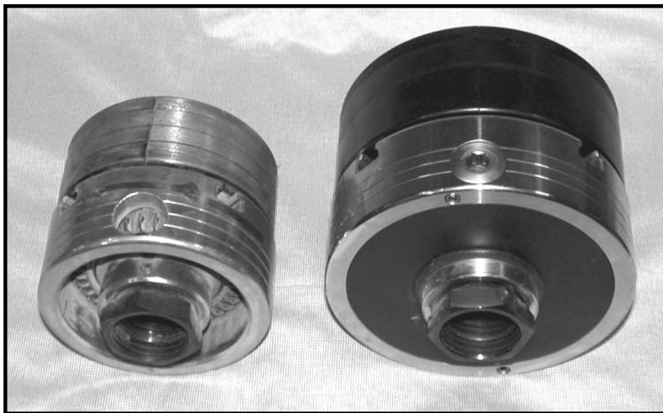
The SuperNova and Titan are shown from the headstock mounting end of the chuck. Note the sealed back on the Titan.
