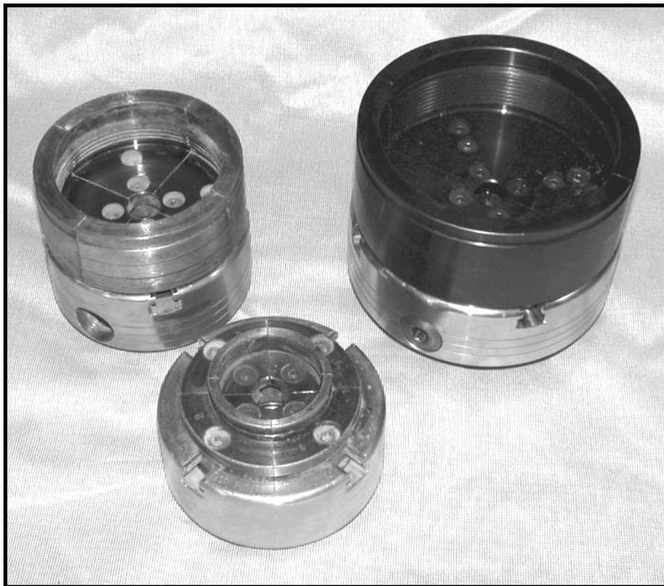
Comparison of SuperNova Chucks to the New Titan (upper right hand corner). The Titan and SuperNova on top are both equipped with Powergrip jaws. Note how much larger the Titan looks.
