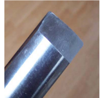
This view shows the actual bevel of the Mario Rodriguez 3-1 Spindle Gouge.
