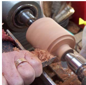
Since both ends of this wood were not true, the next operation was to true the ends.
