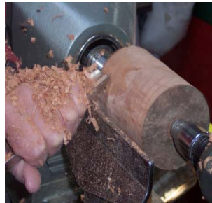
Here I am making the final smoothing cuts on the surface.
