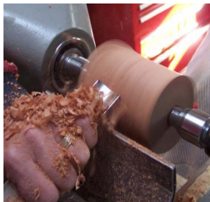
Using the tool for roughing to round.
