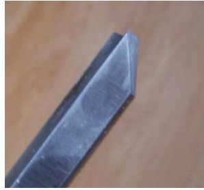
Side view of the Mario Rodriguez 3-1 Spindle Gouge, 1-1/4" wide. The Bevel Angle is 30 degrees a good angle for spindle work.
