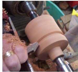
Next operation to perform was try turning a bead with the tool. This was tricky but doable.
