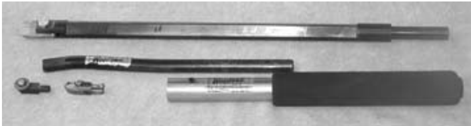
Two Shear Scrapers: Kelton Tool on Top and the Woodcut tool on the bottom.
